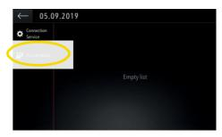
8 To enable Live Navigation Plus activate "Sharing data and vehicle position" and confirm with A.
